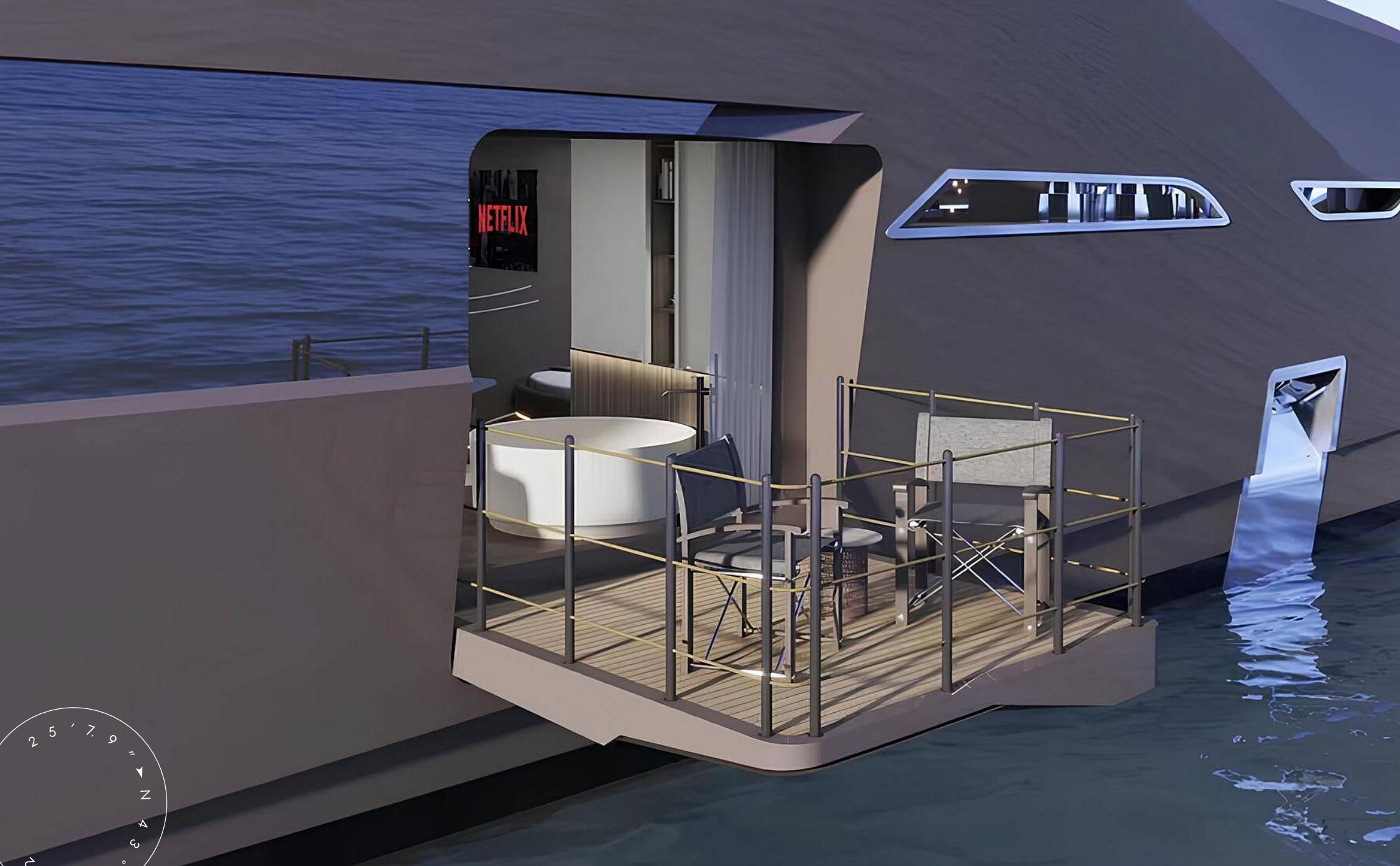
FOLDING STARBOARD BALCONY
